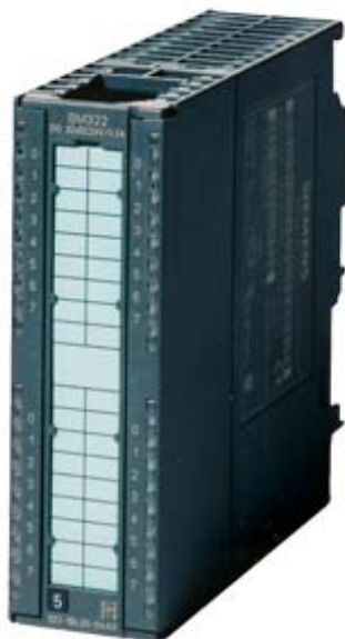
SIMATIC S7-300, DIGITAL OUTPUT SM 322, OPTICALLY ISOLATED, 8 DO (RELAY), 1 X 40 PIN, 24V DC, 120 - 230V AC, 5A WITH INTEGR. SNUBBER F. IND. LOADS
